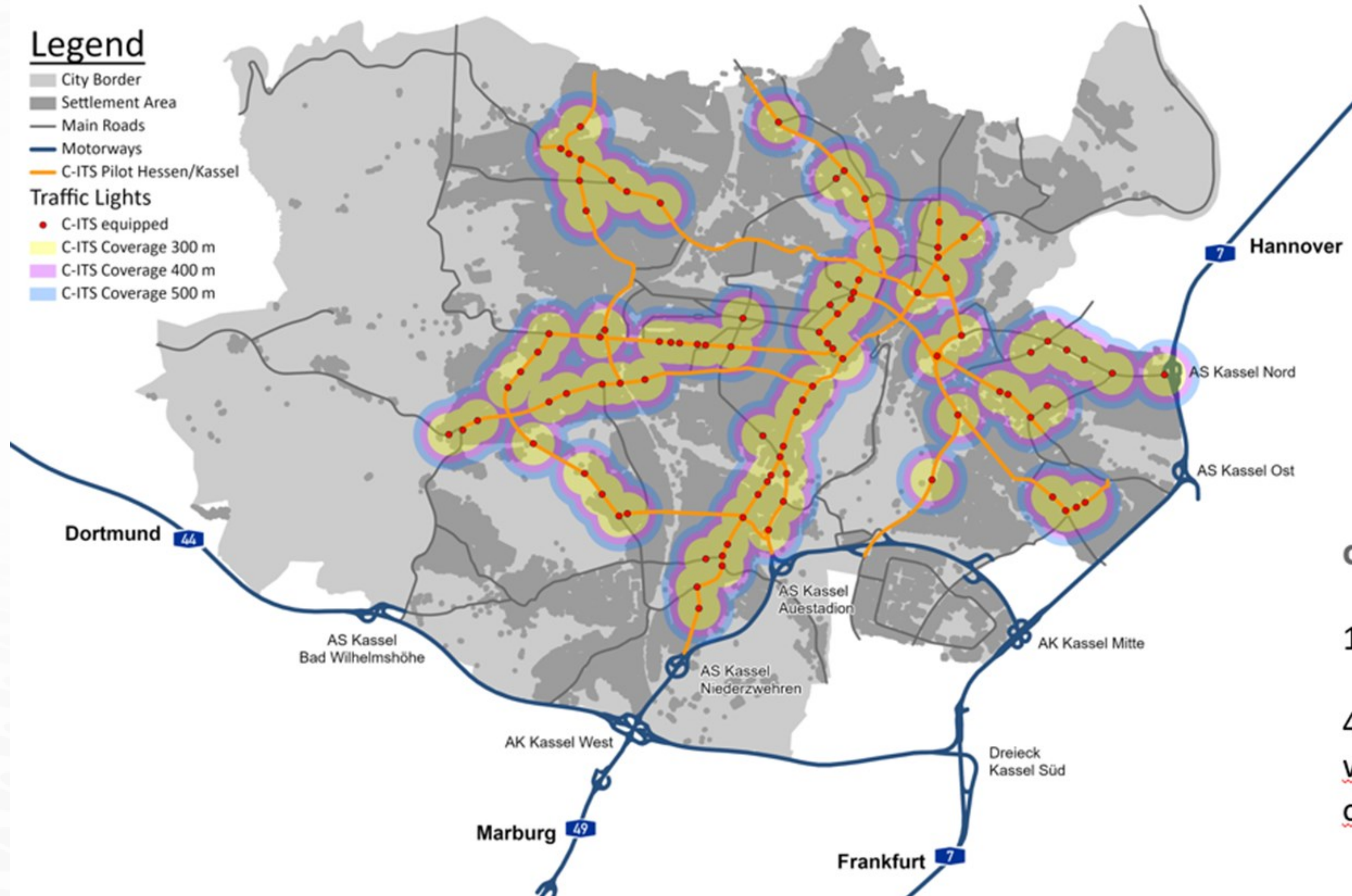
C-ITS equipped traffic light controller with C-ITS coverage (until 07/2023)
